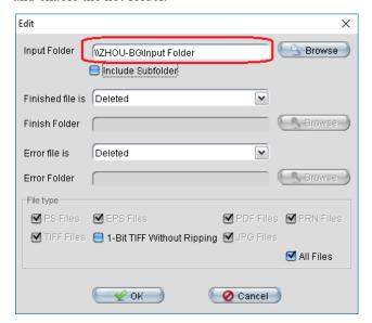
5. Submit the jobs into the shared folder as above pic. In 5 seconds the jobs will be processed by EagleRIP, and the 1-bitTIFF files will be saved into the folder as in step 2.
