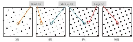
• Miracle Cell technology: Increase ink density of shadow in flexo printing, this special technology greatly improves the shortage of insufficient solid ink of flexo printing.
